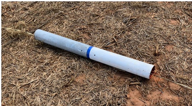
Figure 2: Forward and Central Airframe at Recovery Site
