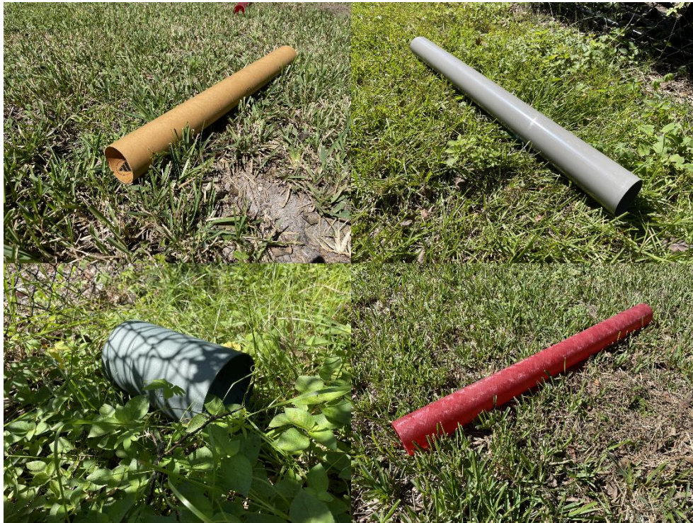
Figure 67: Airframe Samples Following Impact Resistance Test
