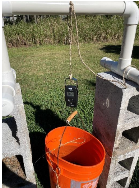
Figure 81: Measurement of Weight at Tensile Failure
