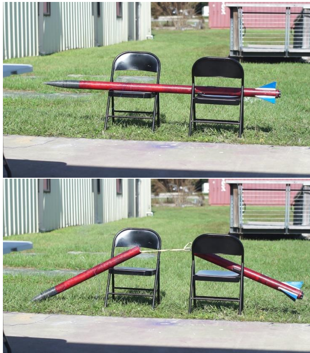
Figure 97: Failed Drogue Ejection
