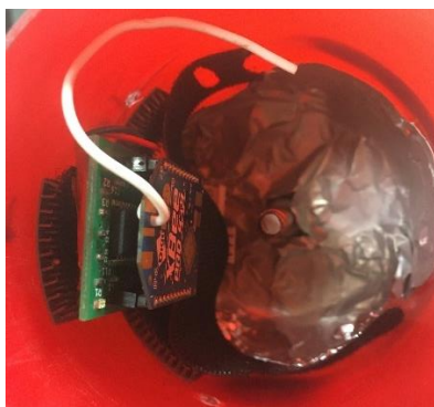
Figure 33: GPS Transmitter in Launch Vehicle
