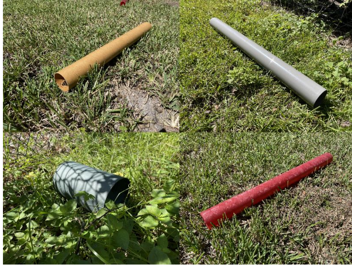
Figure 85: Phenolic (top left), Quantum Tube (top right), Blue Tube (bottom left), and G-12 Fiberglass (bottom right) Airframes After Drop Test
