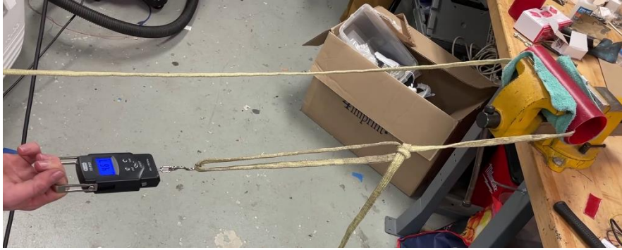
Figure 86: Airframe Material Zippering Resistance Test
