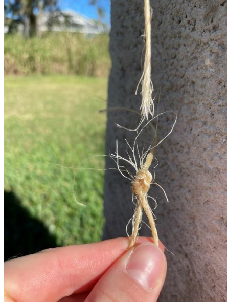
Figure 80: Failure at Knot Location
