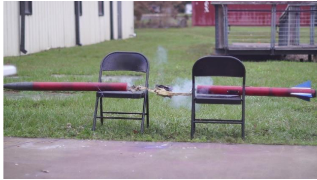
Figure 99: Successful Drogue Ejection
