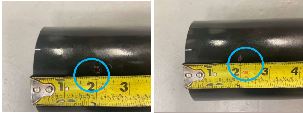
Figure 17: Rivet (left) and Shear Pin (right) Holes in Forward Airframe
