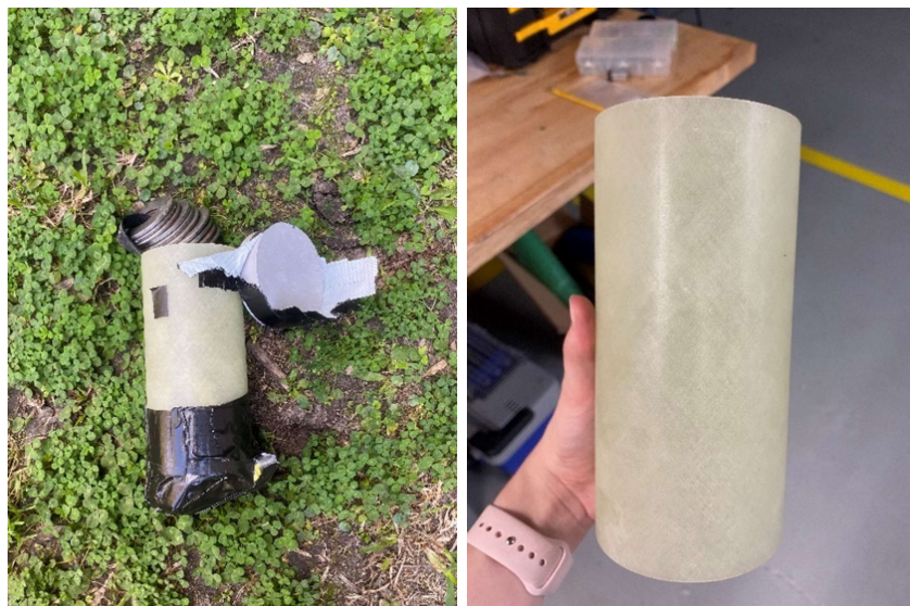
Figure 128: Airframe on Ground After Drop (left) and Airframe After Drop Test (right)
