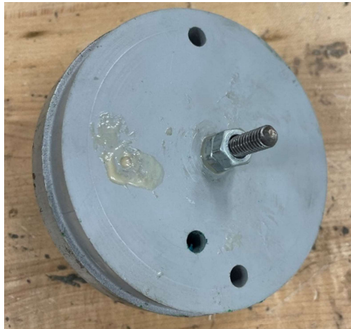
Figure 5: As-built Bulkhead and Epoxied Eyebolt
