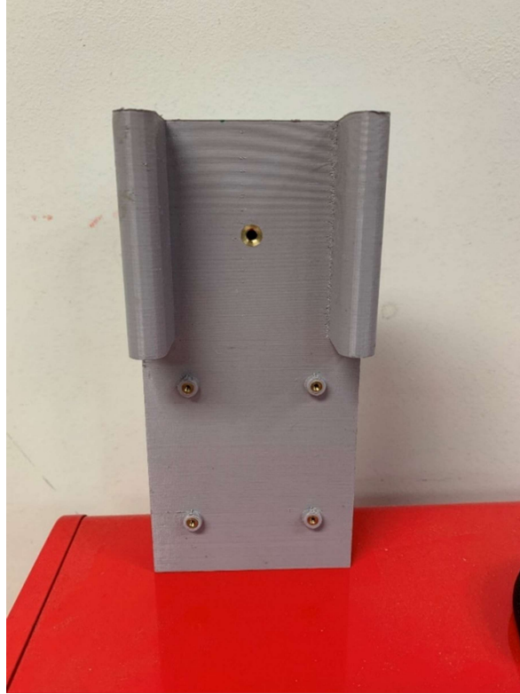
Figure 87: Threaded Inserts Installed on Payload Sled
