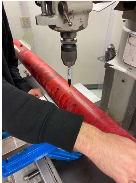
Figure 56: The Setup Used to Align the Forward and Aft Rail Button Locations.
