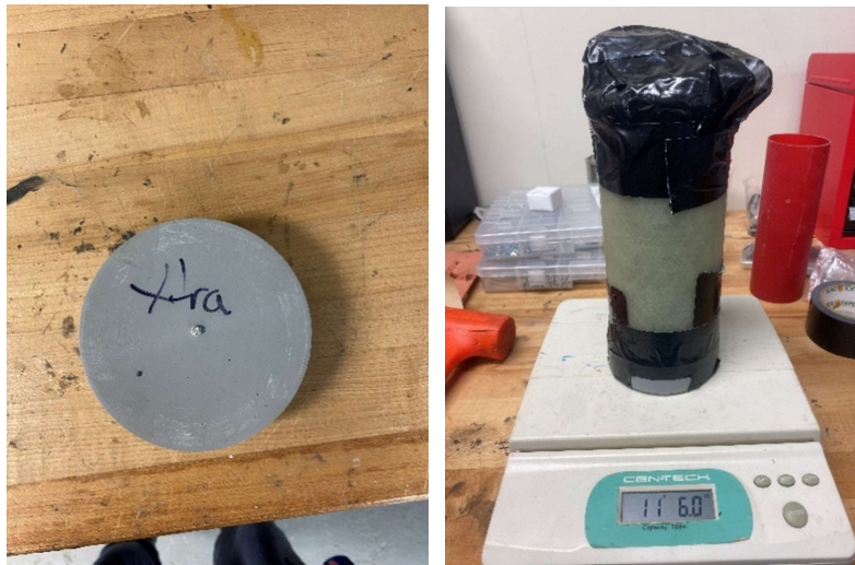
Figure 129: Bulkhead Before Drop Test (left), Total Weight of Bulkhead, Airframe, and Ballast (right)
