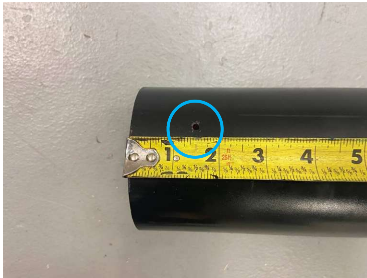
Figure 45: Rivet Hole in Aft Airframe
