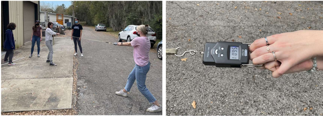
Figure 141: Inducing Force on the Recovery Harness (left) and Force at Which it Was Pulled (right)
