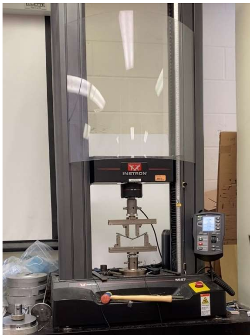
Figure 123: Crosswise-Fiber Specimen Loaded in the Instron
