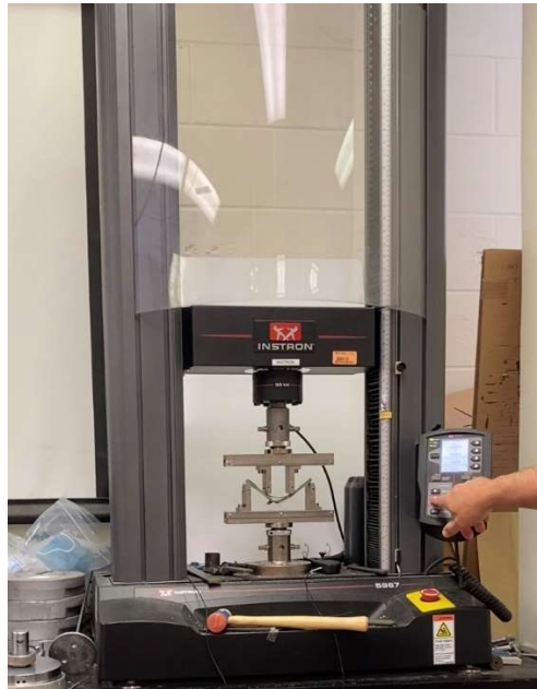
Figure 122: Lengthwise-Fiber Specimen Loaded in the Instron
