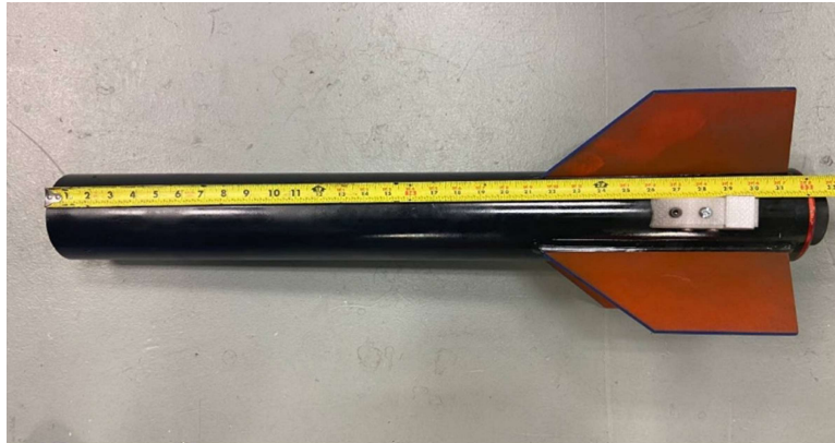
Figure 54: As-Built Lower Aft Airframe Assembly
