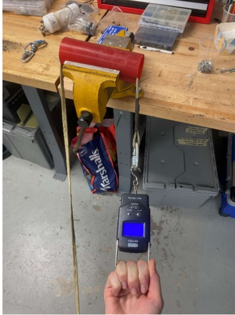
Figure 142: Inducing Zippering Force on Airframe
