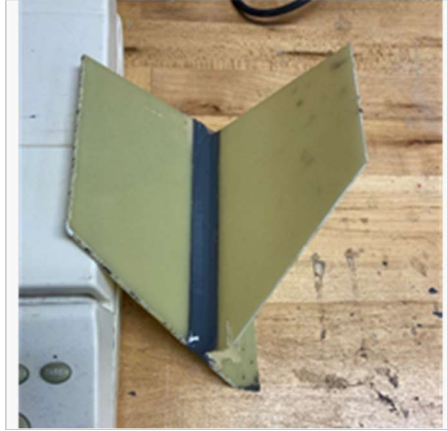
Figure 144: JB Weld Density Inspection
