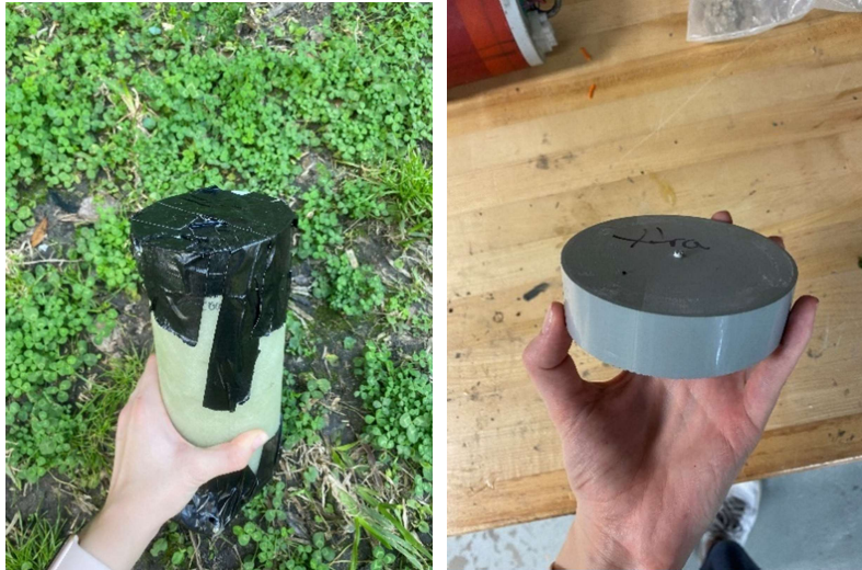
Figure 130: Bulkhead on Ground After Drop (left) and Bulkhead After Drop Test (right)
