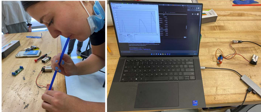
Figure 135: Stratollogger Functionality Test Being Performed (left) and Curve Produced (right)
