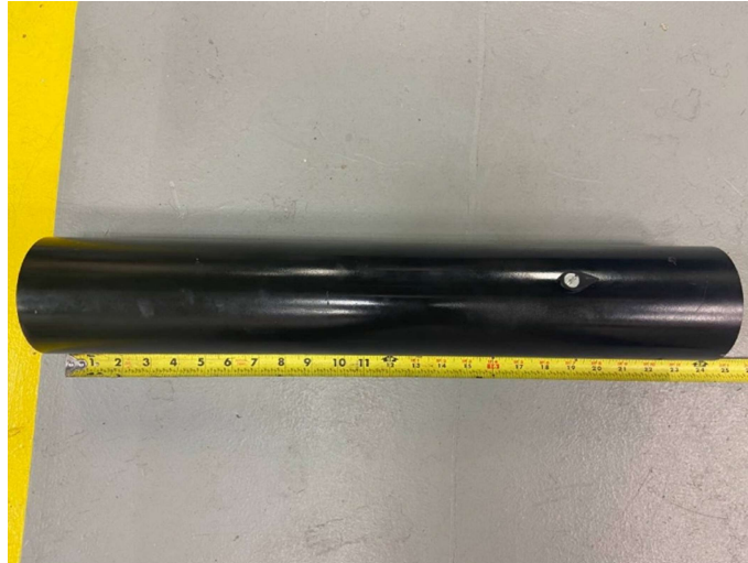
Figure 57: As-built Upper Aft Airframe
