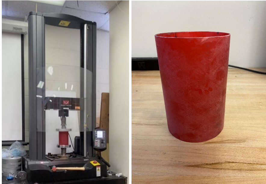
Figure 126: Airframe Specimen Loaded in Instron (left) and Specimen After Compression Test (right)
