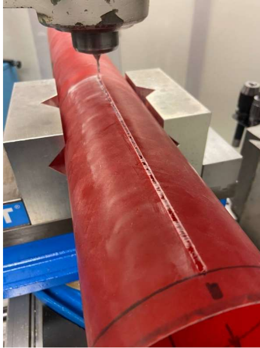
Figure 44: Fin Slot in Aft Airframe After One Pass of the End Mill
