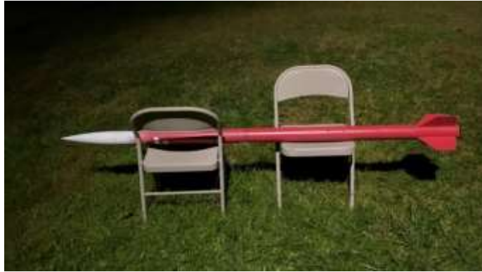
Figure 75: Subscale Drogue Ejection Demonstration Setup
