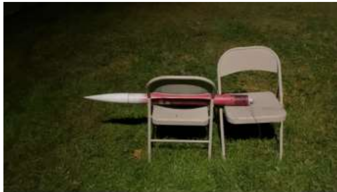
Figure 73: Subscale Main Ejection Demonstration Setup
