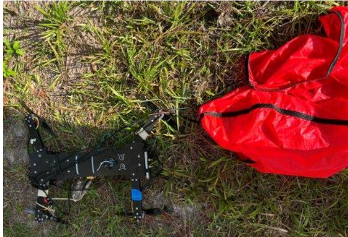
Fig. 39 The quadcopter and its parachute after deploying from the launch vehicle and container.
