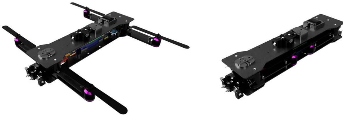
Fig. 17 Stowed (left) and flight configuration (right) of the quadcopter.
