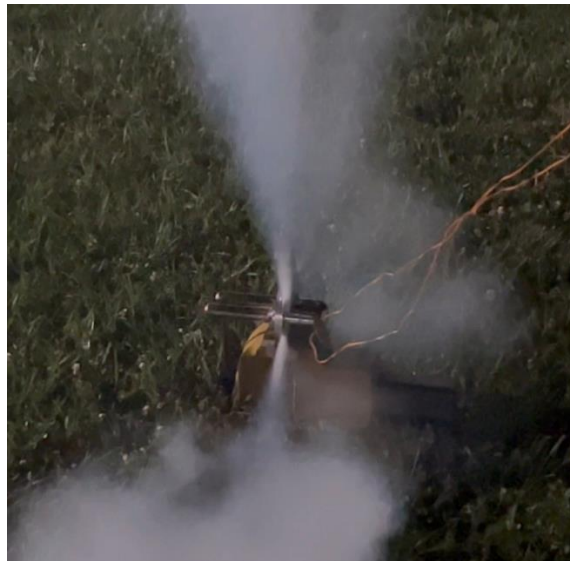
Fig. 34 The CO 2 ejection system is being held by the vise (yellow). The expanding CO 2 gas from the punctured cartridge can be seen as white gas. This happened in less than one second. The visual was captured from a slowed down recording of the test.
