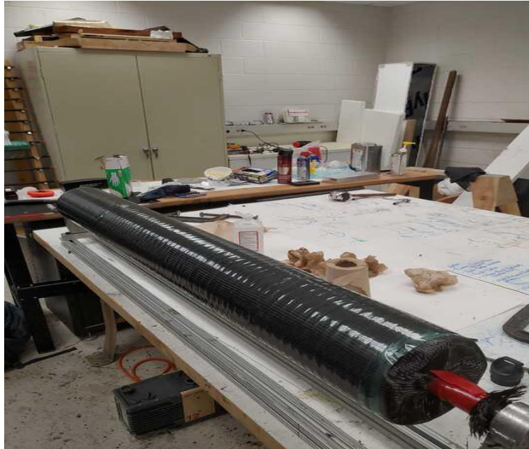
Fig. 8 Layup after tape wrapping on polycarbonate mandrel.
