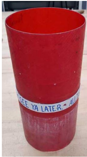
Fig. 11 Avionics Bay coupler with the Switch band epoxied in place.
