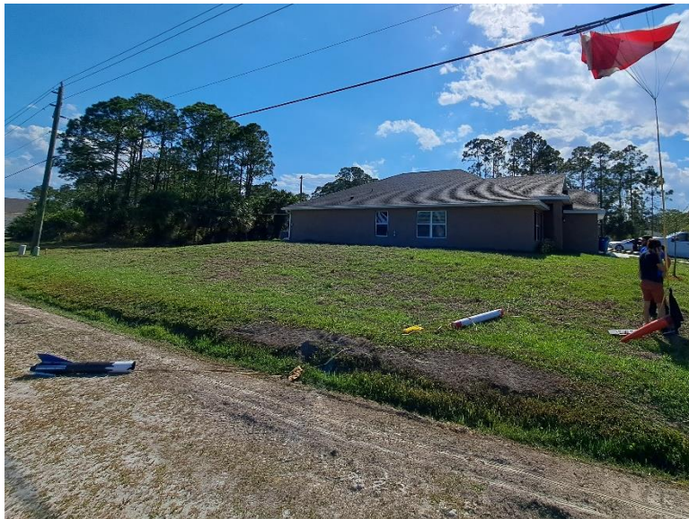
Fig. 36 The recovery site shows the launch vehicle with both sections fully separated. The main parachute was caught in a power line, however the launch vehicle and payload were fully recovered.
