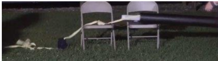
Fig. 38 Ejection testing of the forward airframe with the payload retention system and quadcopter fully assembled. The nose cone successfully sheared off, with the main parachute and its recovery hardware fully deployed. The container with the quadcopter inside (silver box sticking out of the forward airframe) was fully deployed off the 80/20 rail assembly.
