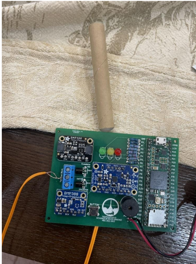
Fig. 47 Flight Computer final design with e-match wired to it.
