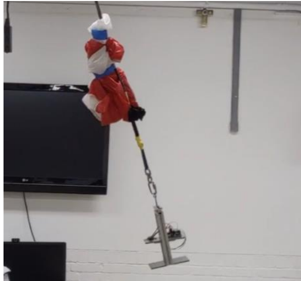
Fig. 24 Experimental setup of the mock-payload. Dummy mass was included to properly replicate moment of inertia of actual payload setup, with angular velocity recorded with a BNO055.
