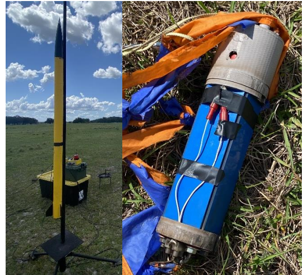
Fig. 43 Left: Kilwin on launch rail prior to launch, Right: Payload landed intact after flight
