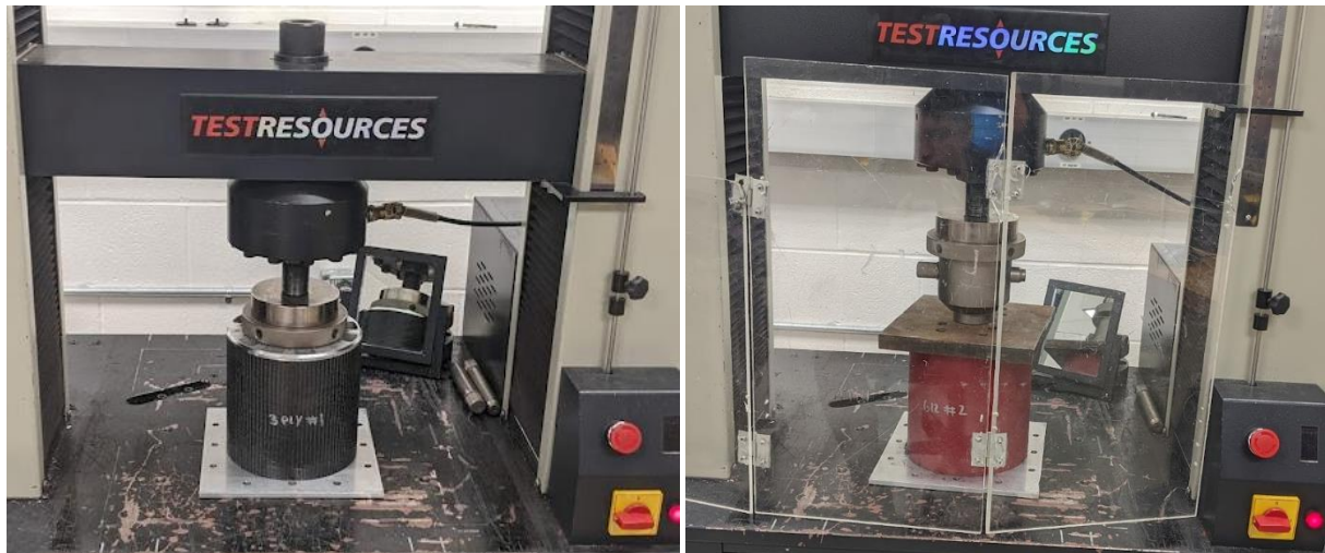
Fig. 40 Left: 3-ply CFRP airframe being tested with the thrust ring. Right: COTS G12 airframe being tested in pure compression
