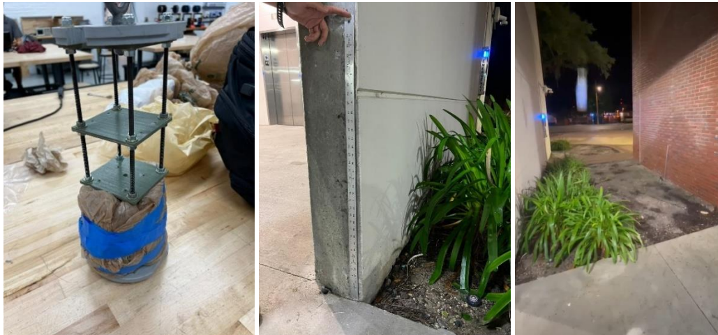
Fig. 41 Left: payload with bottom container filled with sand. The middle section was also filled for the drop test. Middle: ruler set up for speed measurements upon footage review. Right: Payload falling into dirt patch.
